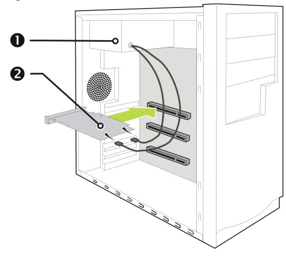
Figure 1–3 Card with Two Power Connections
