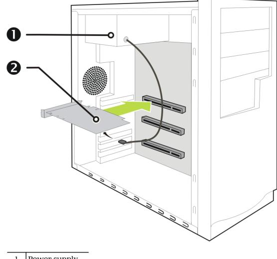
Figure 1-2 Card with One Power Connection
