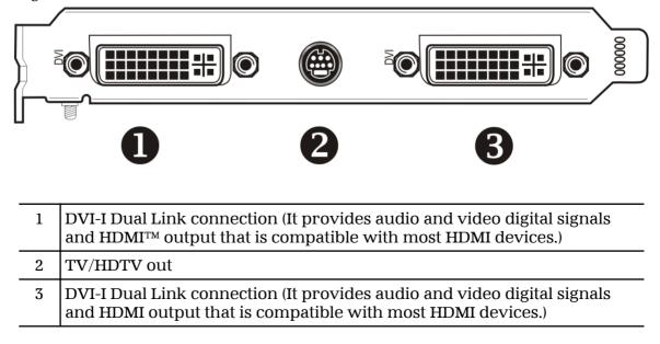
Figure 1-4 ATI Radeon HD 4800 Series Connections
